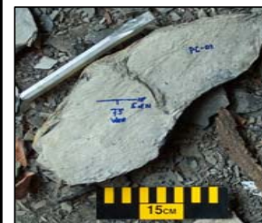
Oriented sample of two deformed mudcrack polygons
